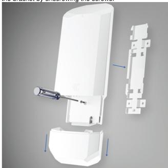
4. Align the OTD500 with the bracket and press it downward until the OTD500's housing is locked into place on the bracket. This locking should close a gap of about 10 mm, or 0.39 inches.
